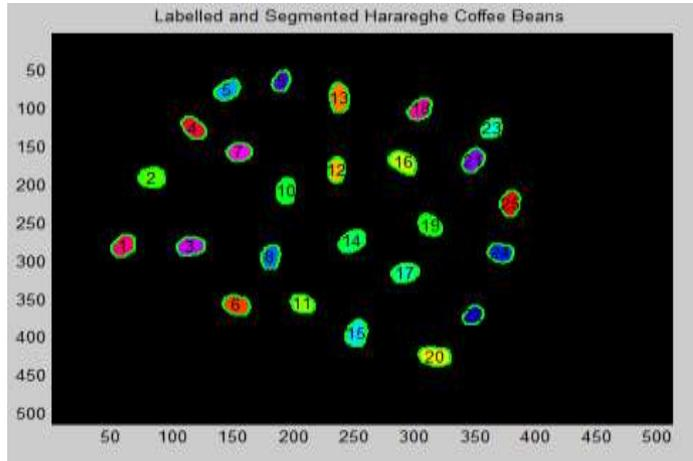
Figure 2. Segmented and labeled Hararghe coffee beans using automatic thresholding.
