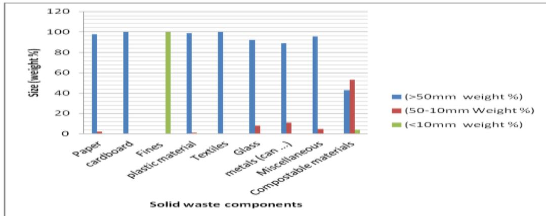
Figure 50. Particle size distribution.
