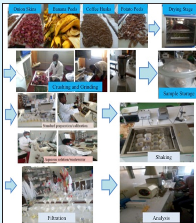
Figure 1: The preparation procedure for low=cost adsorbents from agricultural wastes
